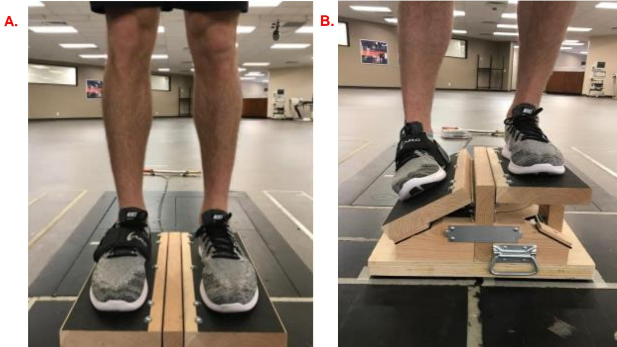
**Figure 1:** For the sudden inversion event, participants stood with feet shoulder width apart on a wooden platform that contained trap doors under each foot (A). Then, a researcher randomly dropped one of the trap doors, causing the ankle to invert 30° (B).
